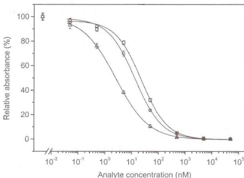
**Figure 2.** Comparison of normalized calibration curves of direct-competitive ELISA with the mutant GlnL89Glu/ValH37Ile/GluL3Val for atrazine (O), iPr/Cl/C6 (Δ) and H/Cl/C6 (□) using the tracer iPr/Cl/C6-HRP. (Dilution of the enzyme tracer: 1 : 5000; error bars: range of triple determination)
