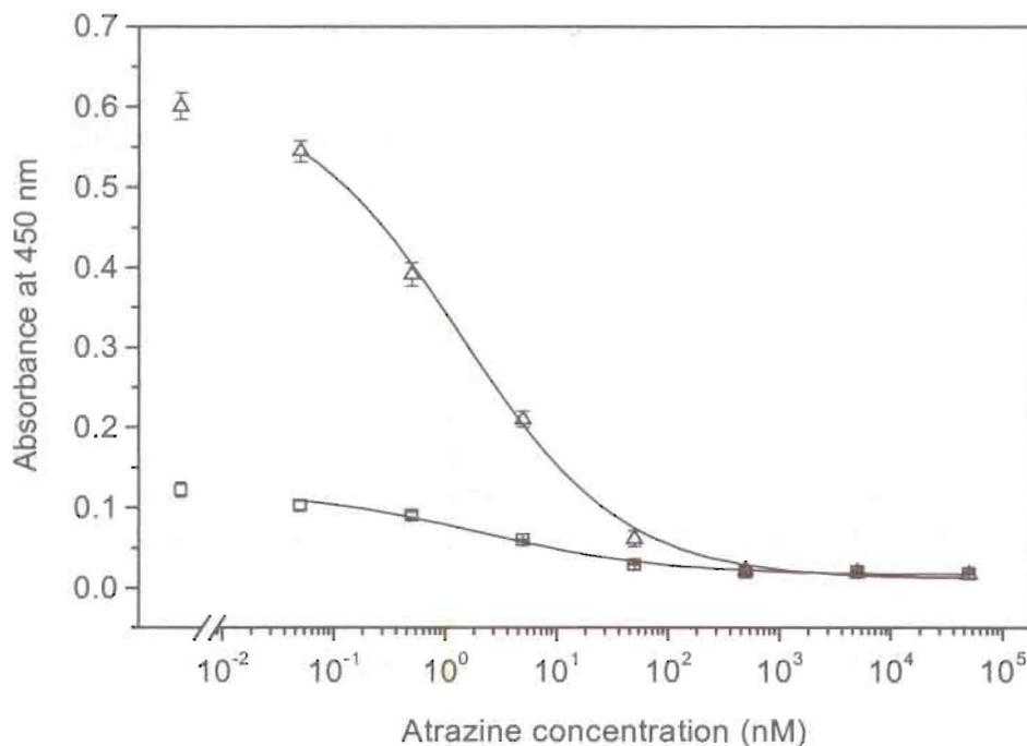
**Figure 3.** Comparison of the absorbance at 450 nm in direct-competitive ELISA for atrazine obtained with the wild-type K411B (□) and the mutant GlnL89Glu/ValH37Ile/GluL3Val (Δ) using the tracer iPr/Cl/C6-HRP. (Dilution of the enzyme tracer: 1 : 5000; error bars: range of triple determination)
