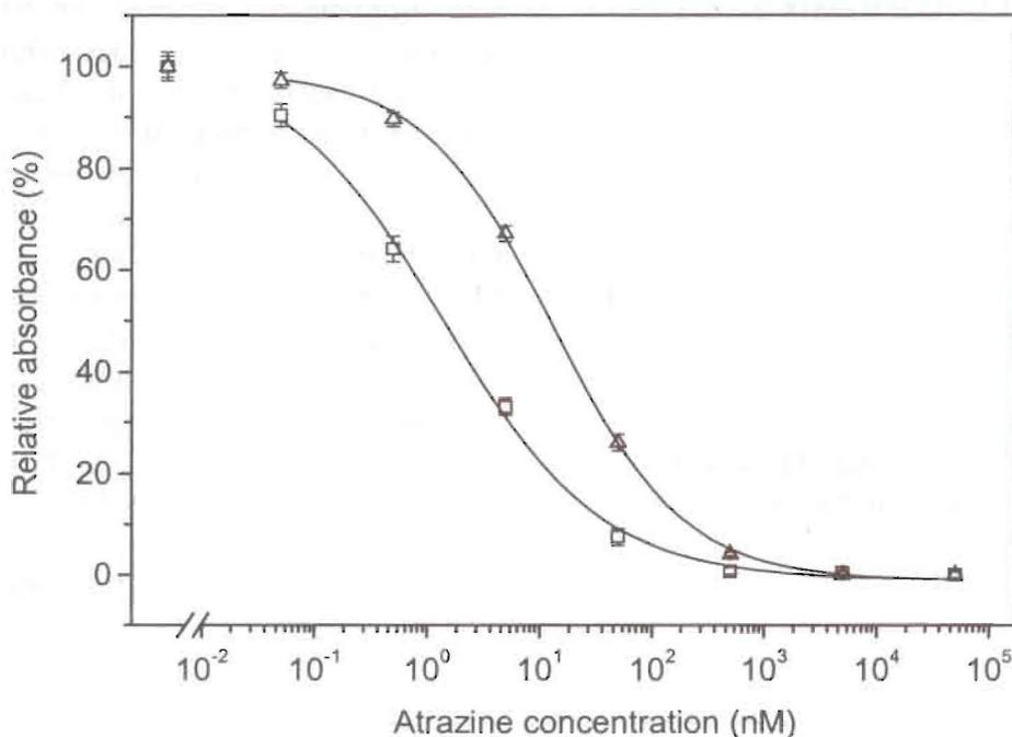
**Figure 4.** Comparison of normalized calibration curves of direct-competitive ELISA for atrazine with the mutant GlnL89Glu/ValH37Ile/GluL3Val using the tracer H/Cl/C6-HRP (□) and iPr/Cl/C6-HRP(Δ). (Dilution of all enzyme tracers: 1 : 5000; error bars: range of triple determination)
